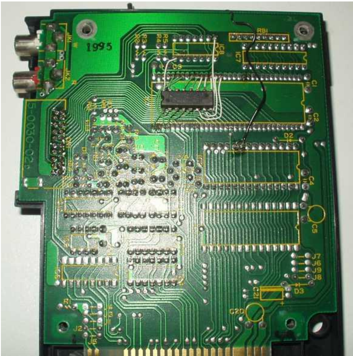
Bottom side of the PCB. Pay attention to the mounting method and orientation of ICs.
